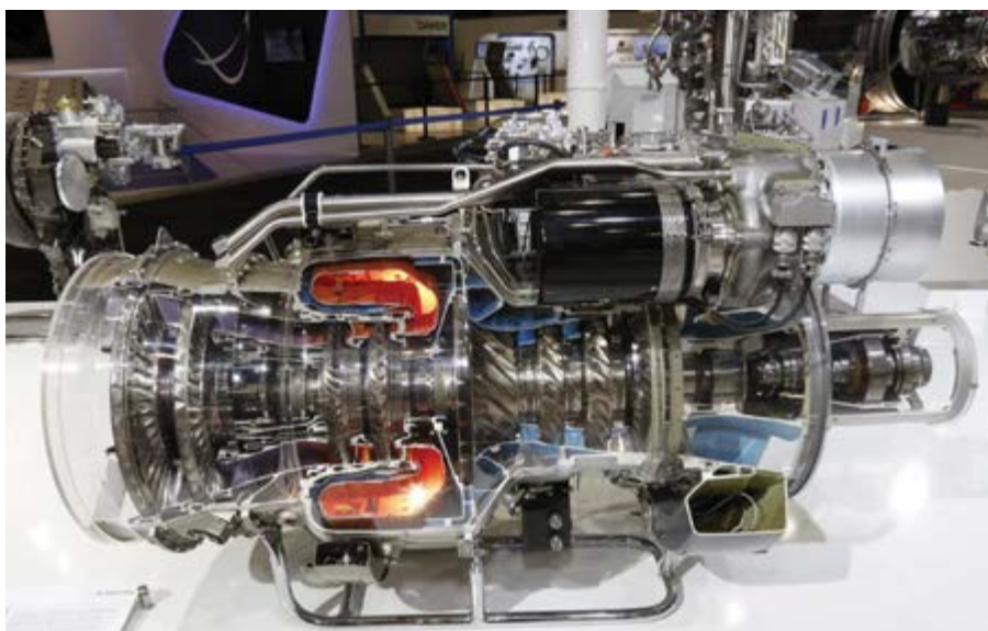
Turbomeca's RTM322 could benefit from technologies developed under the Tech 3000 programme. This sectioned engine shows (right to left) three axial and one centrifugal compressor stages, the annular reverse flow combustor and two-stage compressor and power turbines. (Photo: Turbomeca)
