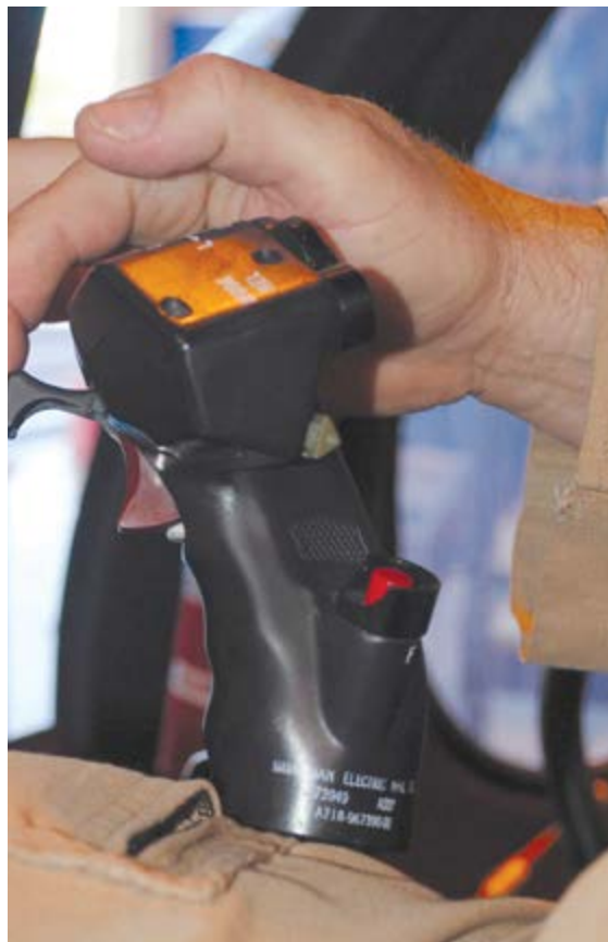
A close-up of the gun trigger on one of the Afghan Air Force's MD 530 gunships. (Photo: author)
