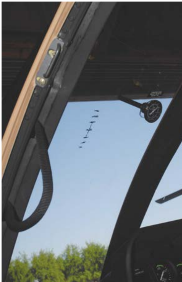
The fire control grease pencil marks on an Afghan MD 530 at MD Helicopters' facility in Mesa, Arizona. (Photo: author)
