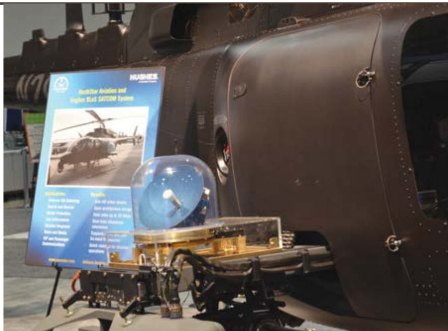
Hughes' HM200 modem weighs 3.6kg and can meet military requirements at up to 30,000ft. (Photo: Hughes Defense and Intelligence Systems Division)
