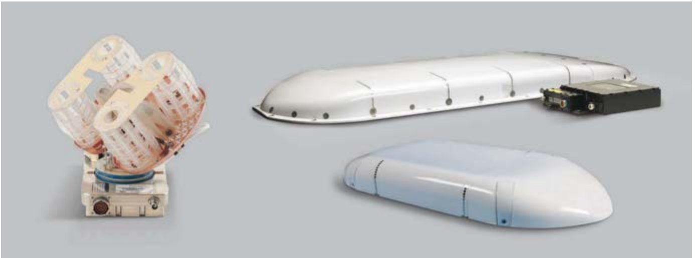
The Aspire 200 SATCOM system has a high-data-rate software package, which allows high-speed and high-bandwidth connections on rotary platforms. (Photo: Honeywell)
